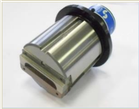
D station punch assembly Standard size 75x15 and 85x15
