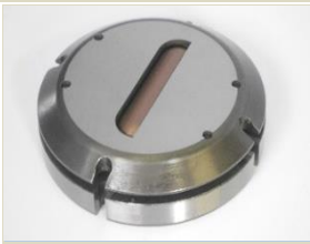
D station die assembly HDP coating
