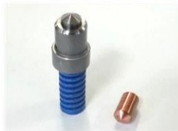
Widia and copper tool UPPER KIT
