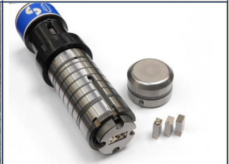
Punch assembly smart style replaceable character
